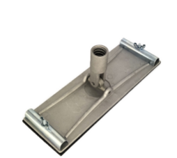
Universal sander block 230 x 80 mm Sturdy die cast aluminium base plate with reinforced ridges to prevent bowing Sponge rubber sandpaper pad allows for softer sanding
